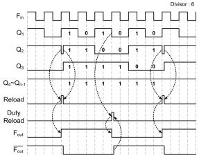
Fig. 3. Timing diagram of the proposed programmable frequency divider.
