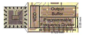
Fig. 6. Die photo of the proposed programmable frequency divider.
