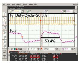
Fig. 8. Output waveforms of the proposed programmable frequency divider when Fin is 700MHz, the input divisor is 20, and the input duty-cycle is 20%.
