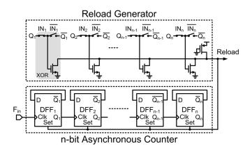
Fig. 4. Proposed programmable counter.
