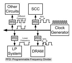
Fig. 1. Applications of the programmable frequency divider with an improved duty-cycle output.
