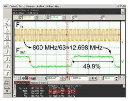
Fig. 7. Output waveforms of the proposed programmable frequency divider when Fin is 800MHz and the input divisor is 63.
