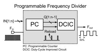
Fig. 2. Proposed programmable frequency divider.
